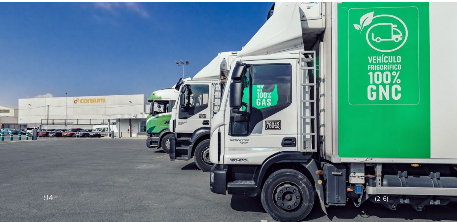
Fleet of compressed natural gas (CNG) lorries
